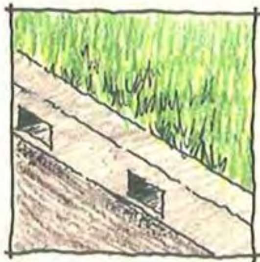
(e) Perforated curb
