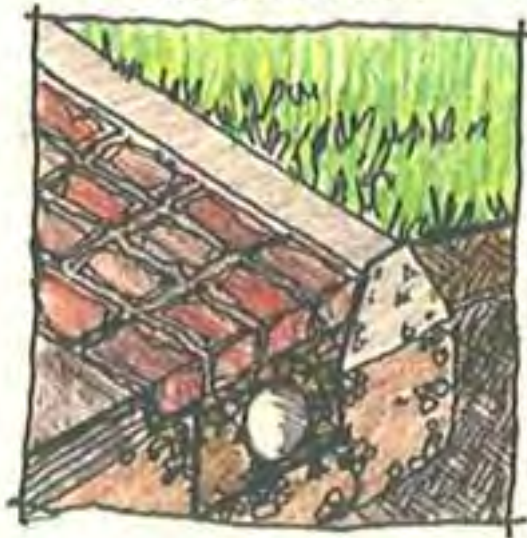
(c) Rumble strip with sediment trench
